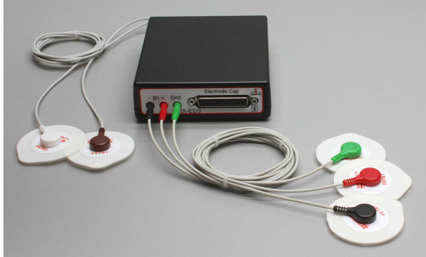
Figure HM-4-S1: The IX-EEG with five EMG lead wires connected.
