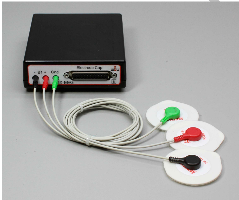
Figure HH-1-S1: The IX-EEG recorder with three lead wires and electrodes connected.
