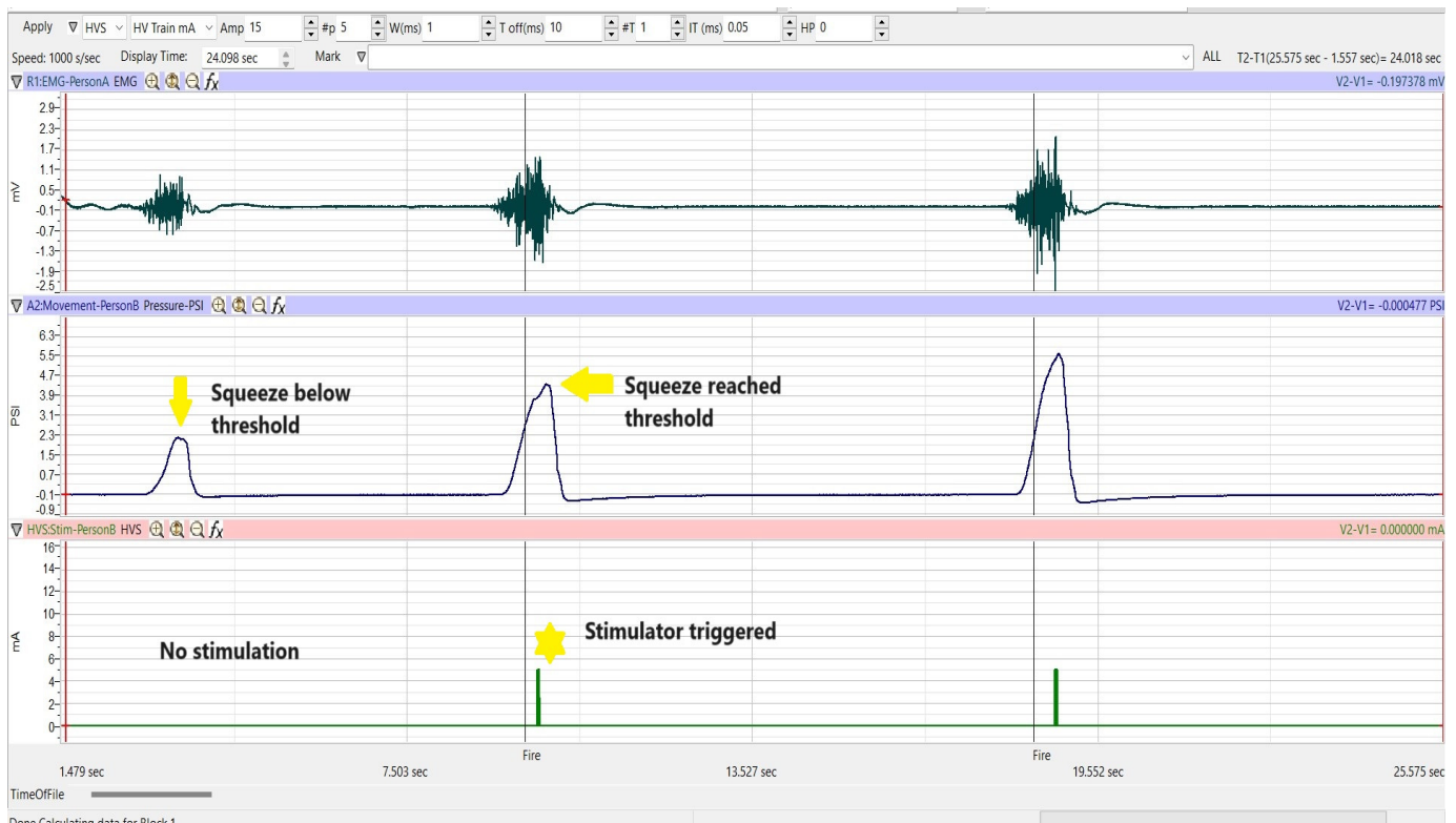
Figure HN-8-L1: A recording showing the person squeezing or flexing and the subsequent firing of the stimulator.
