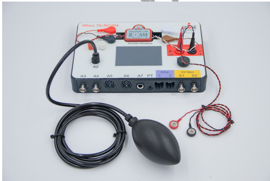
Figure HN-8-S1: IXTA with the FT-220, iWire-B3G and stimulator lead wires for performing the Human to Human Interface lab.
