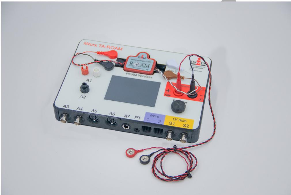
*Figure HN-3-S4: The IXTA with the stimulating electrodes connected correctly.*
