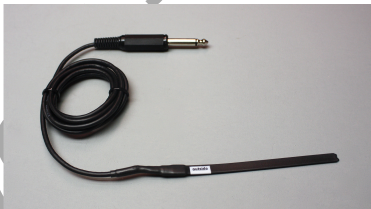
Figure HM-4-S4: The SMT-220 muscle transducer with a label indicating the side of the sensor that faces to the outside.
