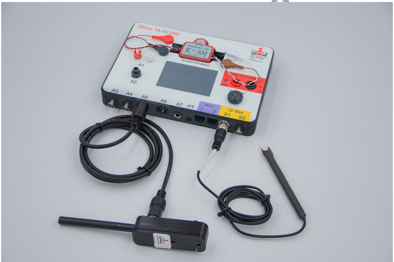
Figure AM-3-S3: The FT-302 force transducer and the A-BST-100 bipolar stimulating electrode connected to the IXTA.
