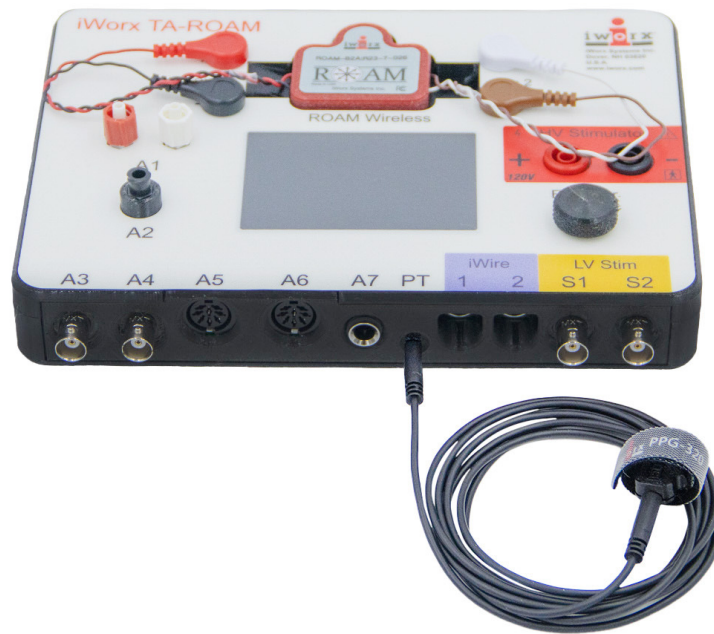
Figure HH-6-S1: The PPG-320 pulse sensor connected to the TA.
