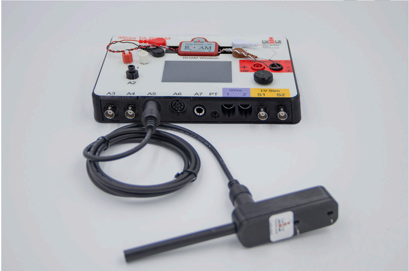
Figure AM-10-S2: FT-302 force transducer connected to IXTA.
