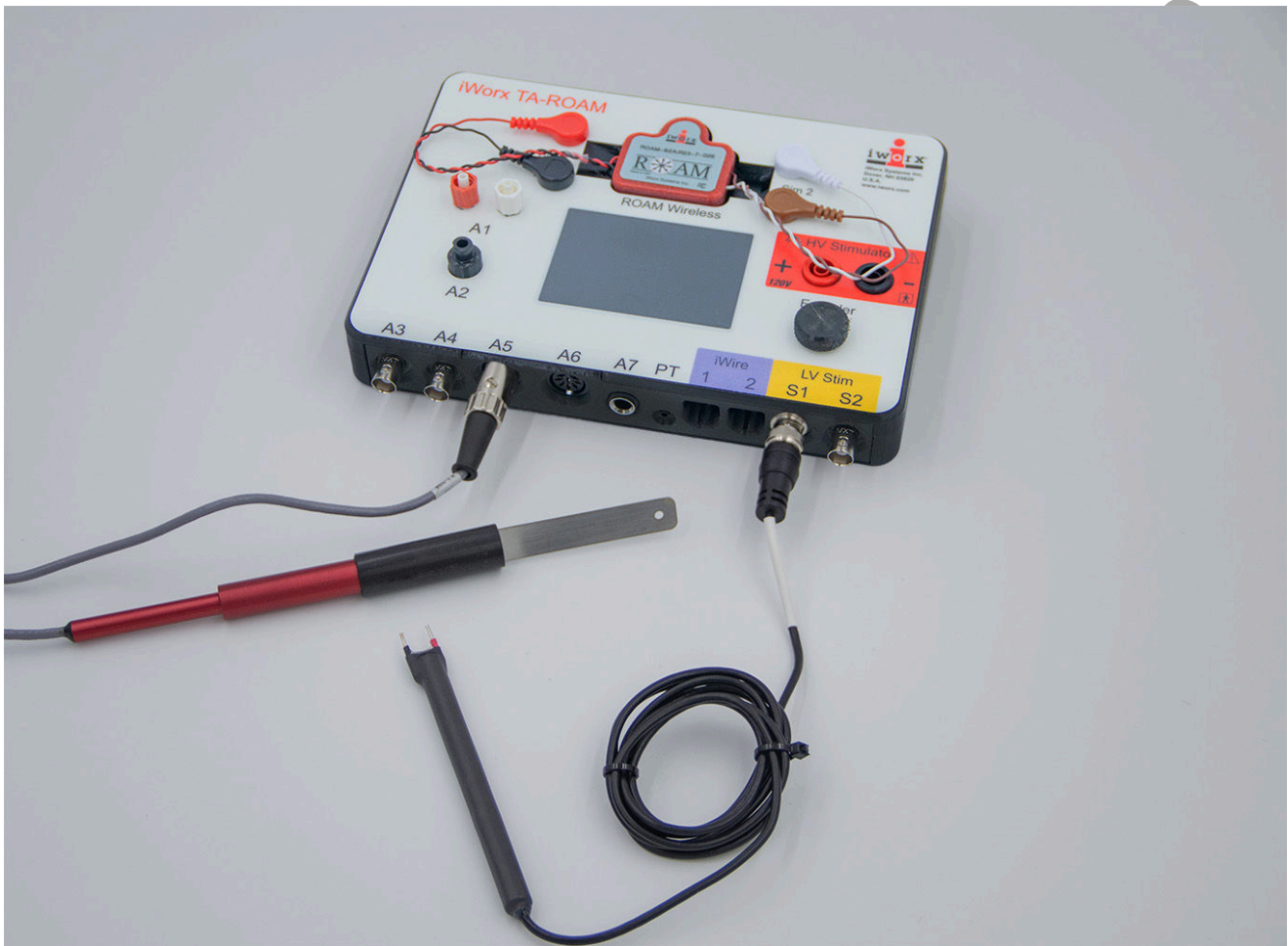
Figure AM-2-S3: The FT-302 force transducer and the A-BST-100 bipolar stimulating electrode connected to the IXTA.
