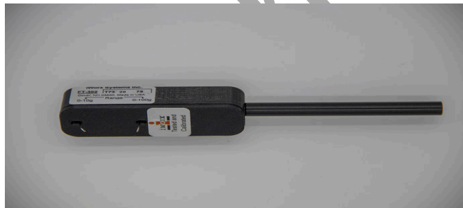
Figure AM-2-S1: The FT-302 force transducer.
