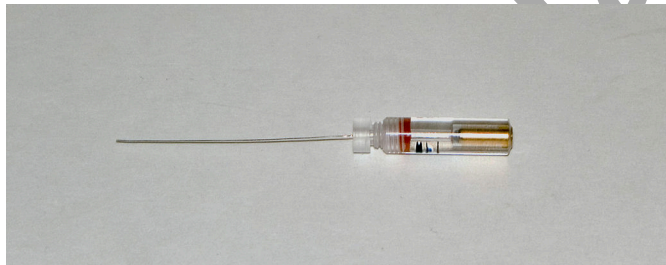
Figure AN-I-S2: The microelectrode holder for the IC-200.
