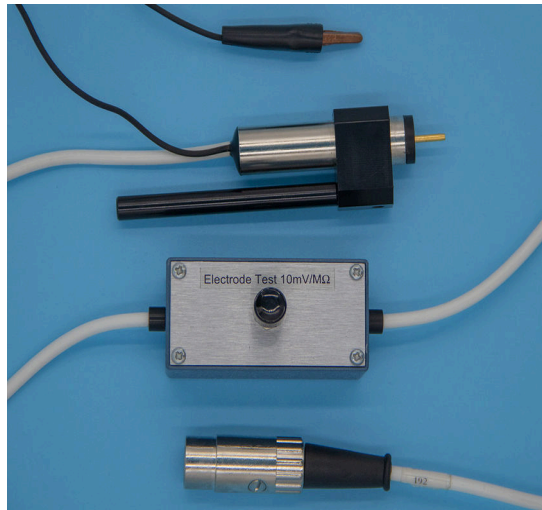
Figure AN-I-S1: The IC-200 intracellular probe.
