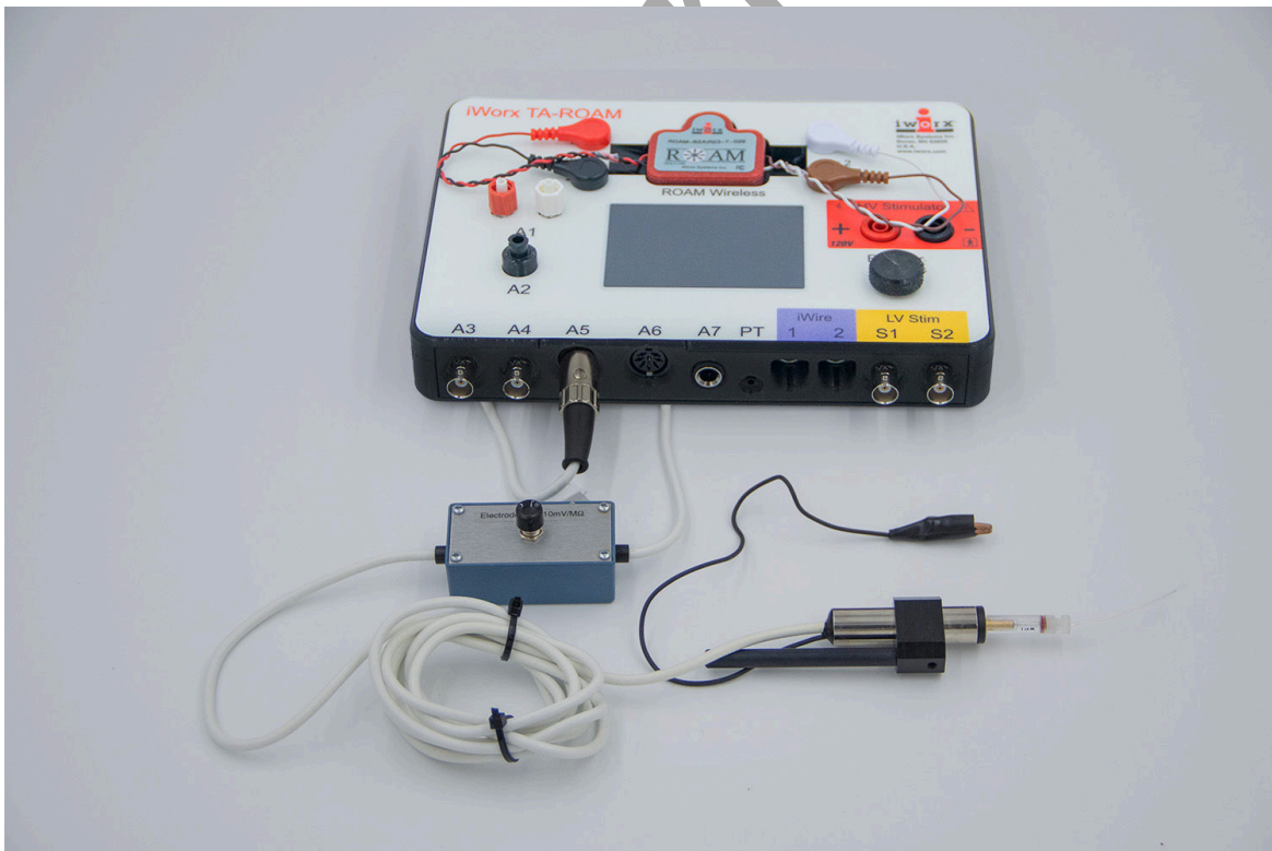
Figure AN-I-S3: The IC-200 intracellular probe with a microelectrode holder connected to an IXTA.
