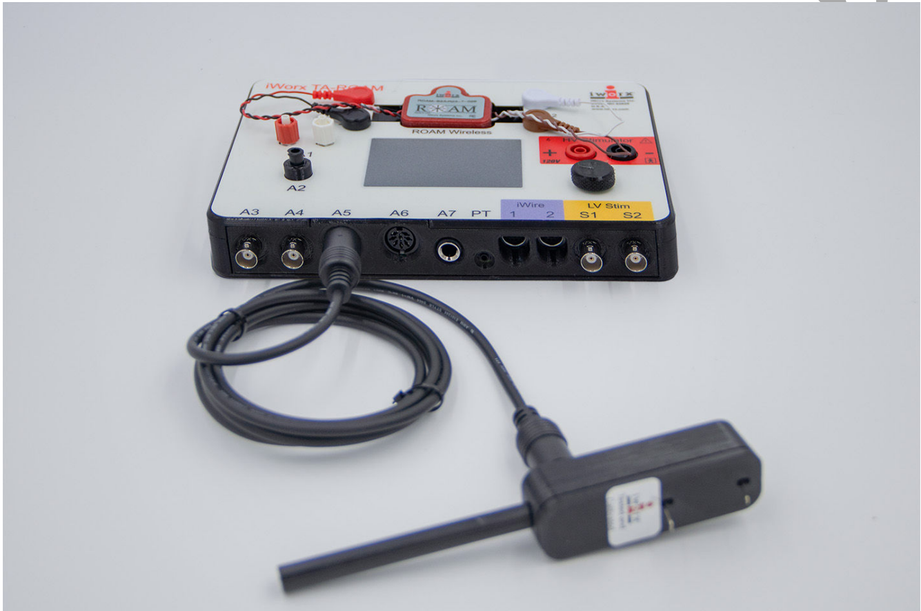
Figure AM-5-S4: The FT-302 dual-range force transducer connected to an IXTA with a male DIN-DIN cable.
