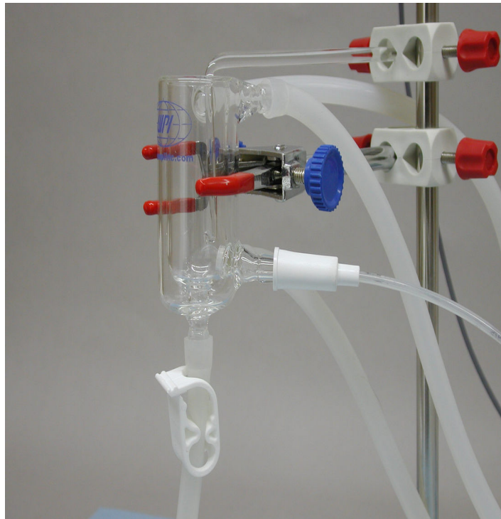
Figure AM-5-S6: 25 ml tissue bath in position for recording tissue tension.
