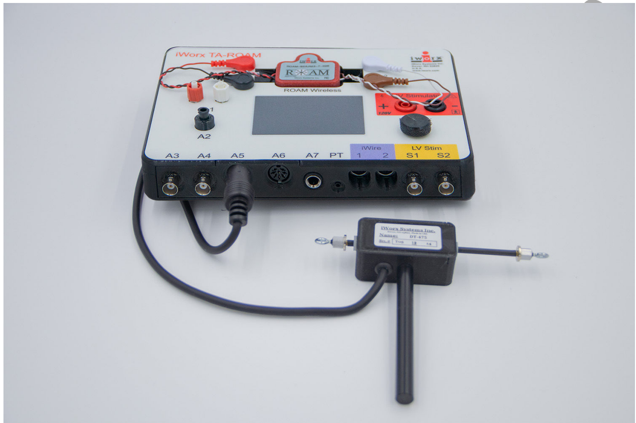
Figure AM-5-S2: The DT-475 displacement transducer connected to an iVortex TA-ROAM system.
