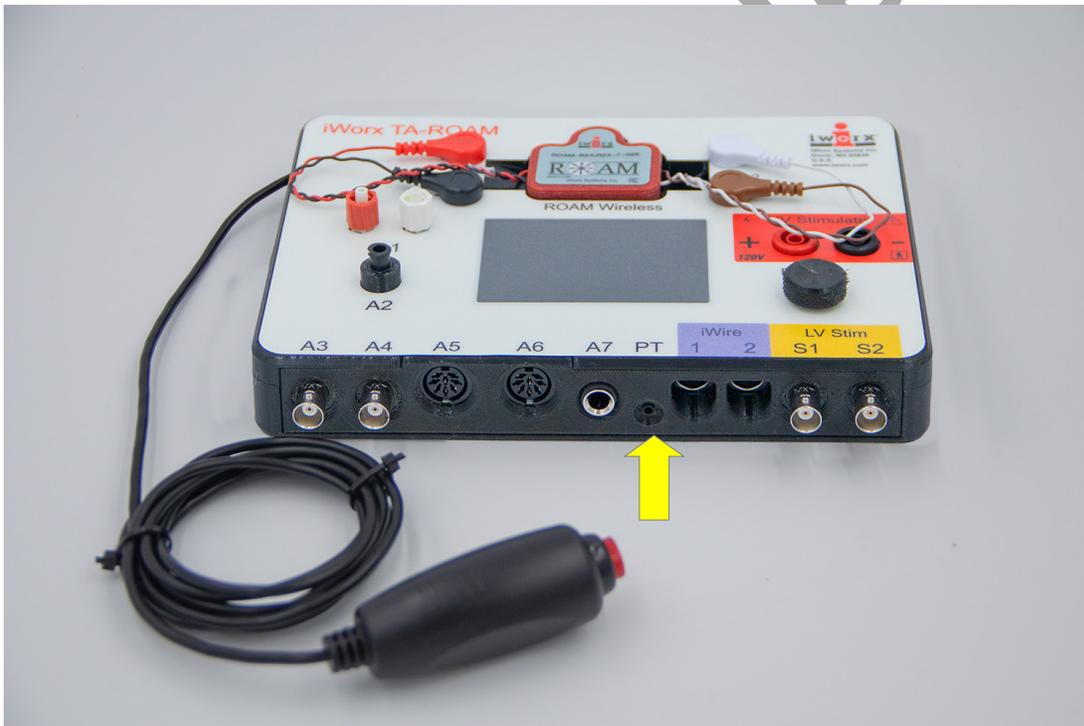
Figure HP-11-S3: The IX-TA shown with the EM-220 plugged into the EM-1 port. The PPG-320 will plug into the PT port.
