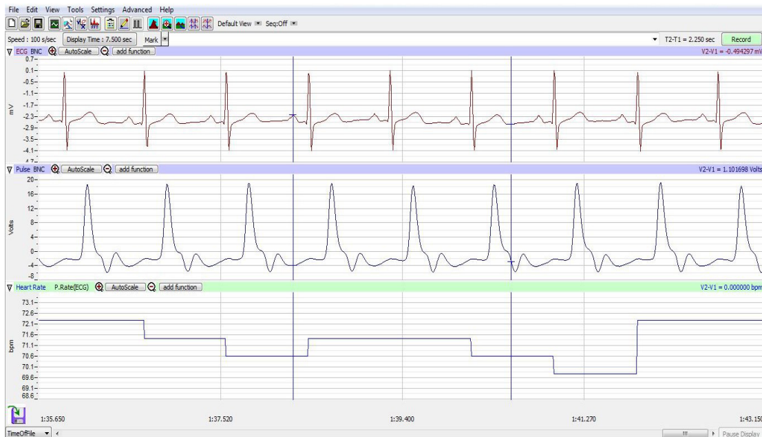
Figure HH-3-L1: ECG, pulse and heart rate displayed on the Main window. The arrow is placed above a dichrotic notch.
