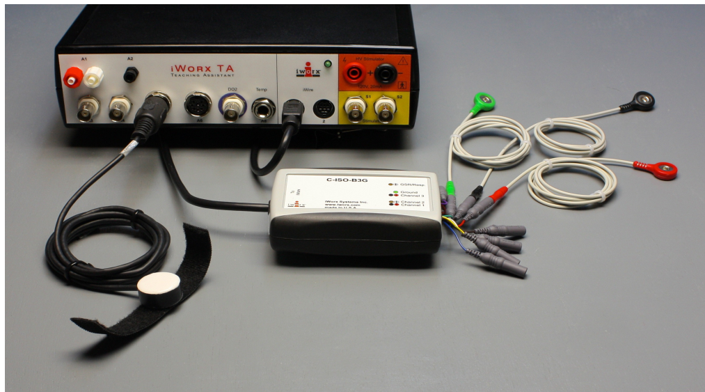
Figure HH-3-S3: The ECG cable and pulse transducer connected to an IXTA.
