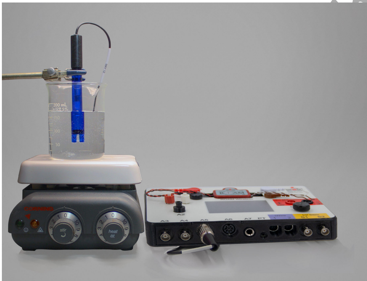
Figure GB-2-S2: The image of the stirrer, pH electrode, and beaker for the calibration of the pH probe.
