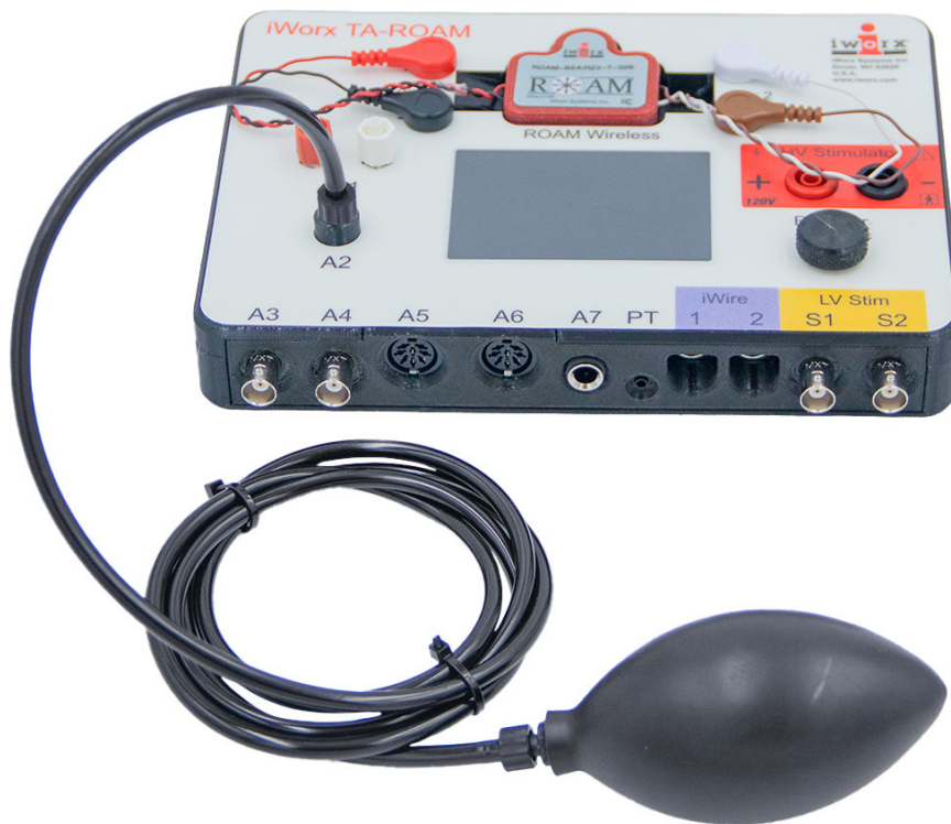
Figure HM-15-S2: The EMG cable and hand dynamometer connected to an IXTA.
