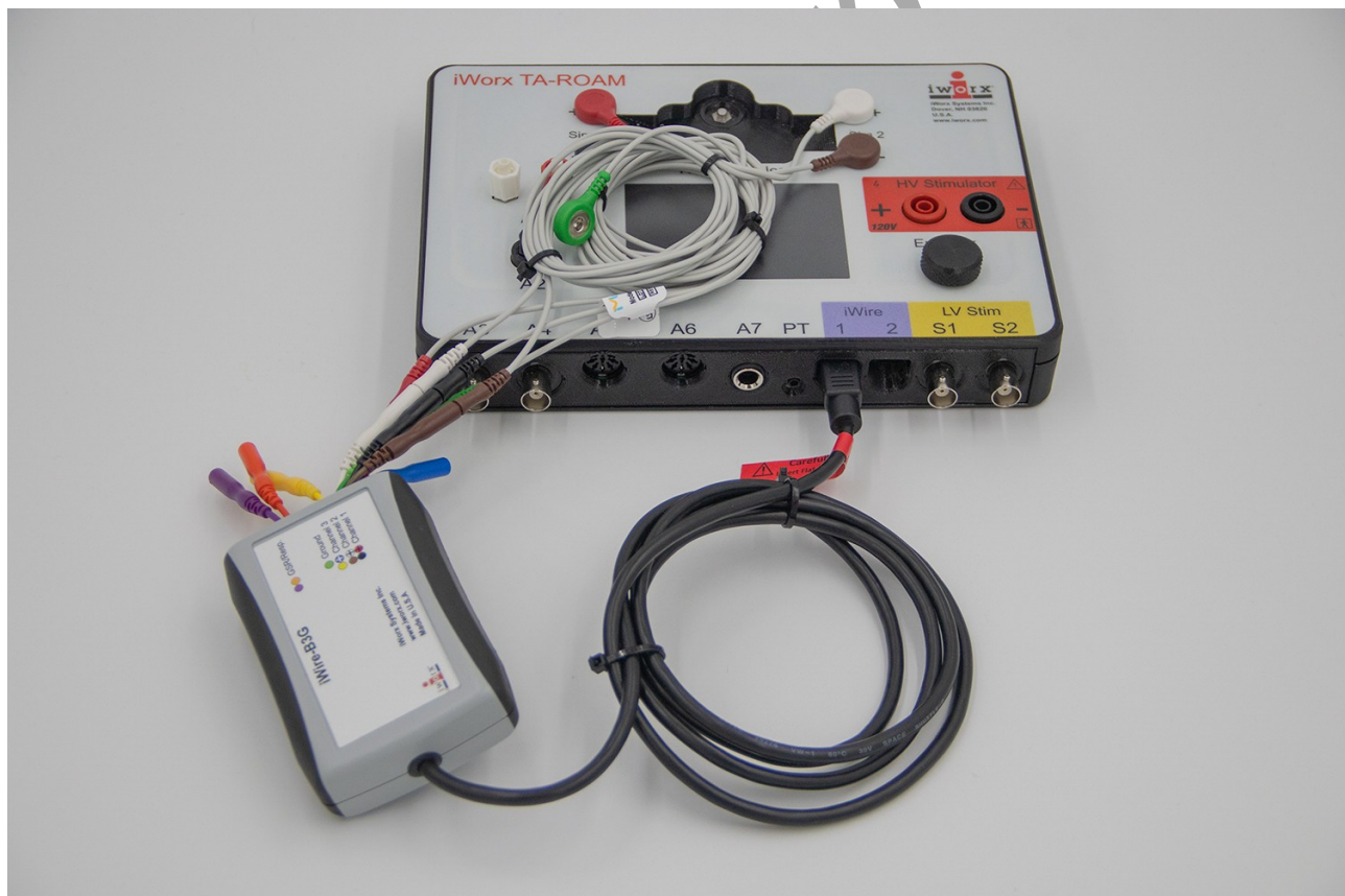
Figure HH-11-S1: The TA with the iWire-B3G connected to the iWire 1 port and the leads connected to the Sim snaps.
