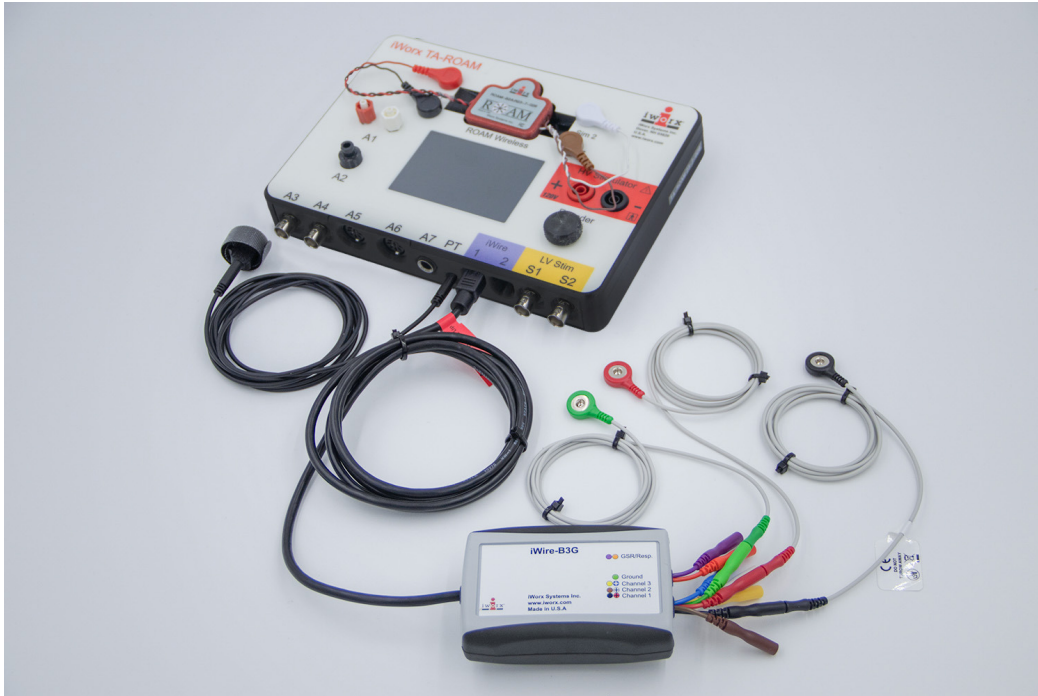
Figure HC-6-S2: The B3G and PPG plugged into the TA.
