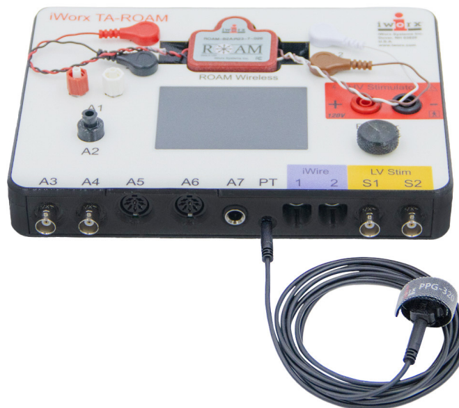
Figure HH-5-S1: The PPG-320 connected to the IXTA.
