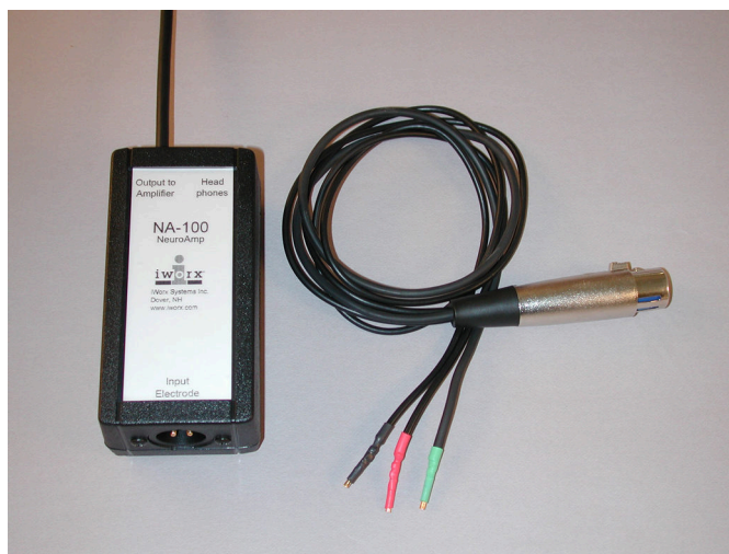
Figure AN-10-S1: The NA-100 NeuroAmp Extracellular Amplifier and input cable.
