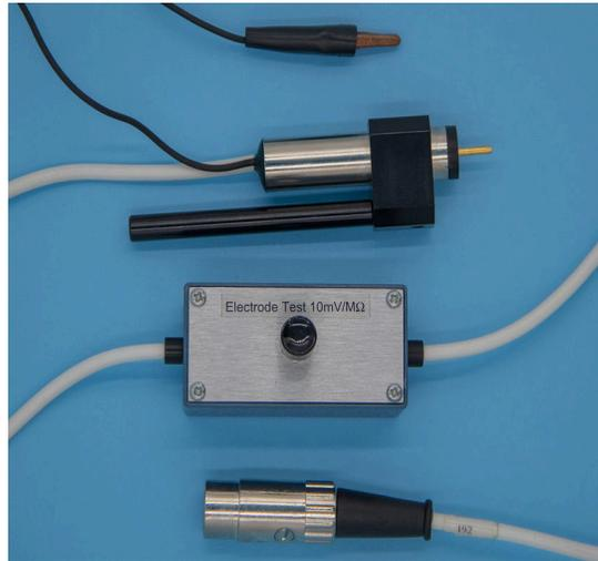
*Figure AN-12-S3: The IC-200 intracellular probe.*
