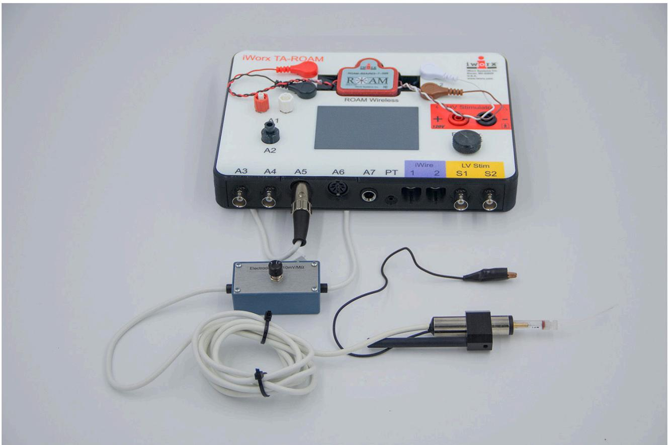
Figure AN-12-S5: The IC-200 intracellular probe with a microelectrode holder connected to an IXTA.
