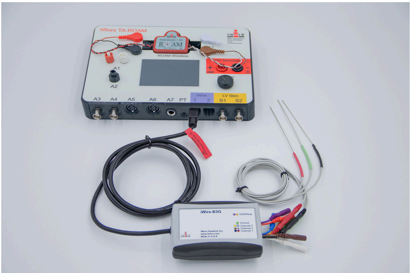
Figure AM-12-S2: The iWire-B3G and C-ISO-F3 leads attached to the IXTA.
