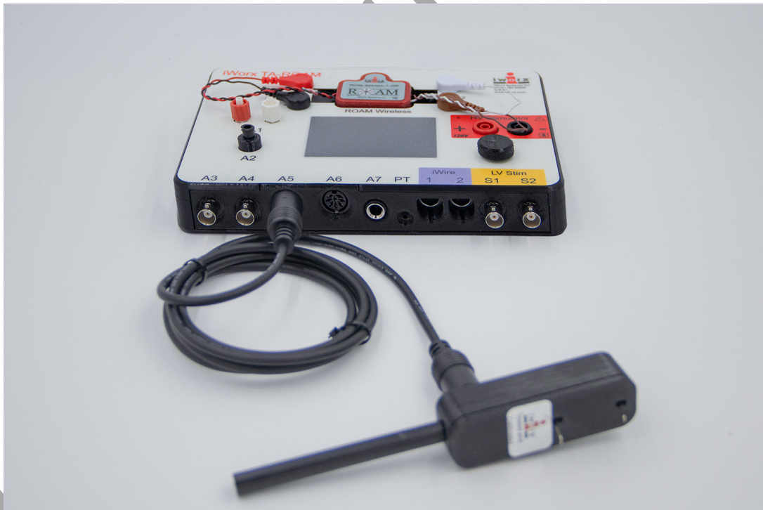
Figure AM-7-S1: The FT-302 force transducer connected to the IXTA.
