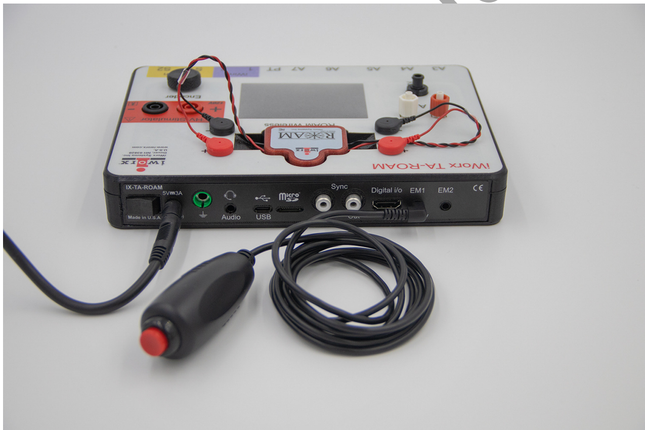
Figure HN-13-S2: The IXTA with the EM-220 event marker.
