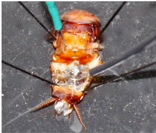
Figure AN-7-S4: The ventral nerve cord situated on the hook electrode and supported by a bed of petroleum jelly.
