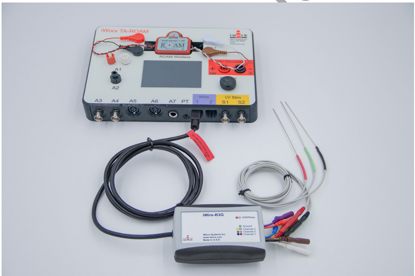
Figure AN-5-S2: The iWire-B3G recording cable attached to the IXTA.
