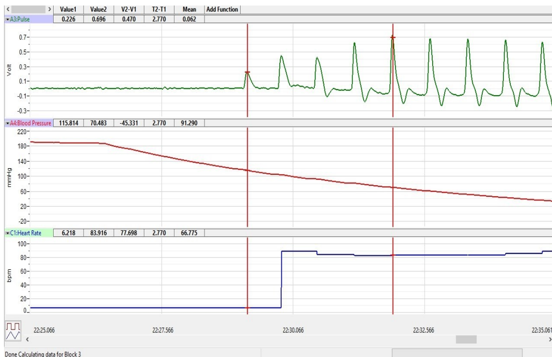
Figure HP-5-L2: The pulse, pressure in the cuff, and heart rate recorded before, during, and after the occlusion of the brachial artery displayed in the Analysis window. Cursors are placed for measuring the systolic and diastolic pressures, which are 115.8 mmHg and 70.4 mmHg, respectively.
