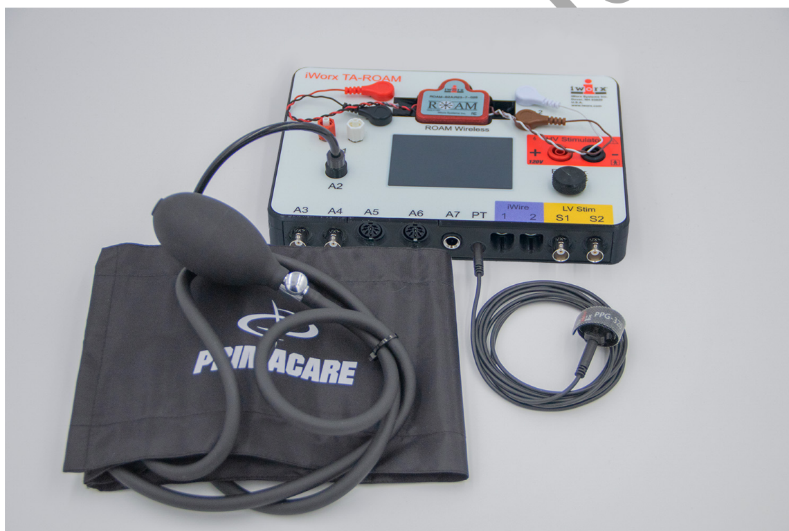
Figure HP-6-S1: The PPG-320 pulse transducer and the BP-220 non-invasive blood pressure transducer connected to the TA.
