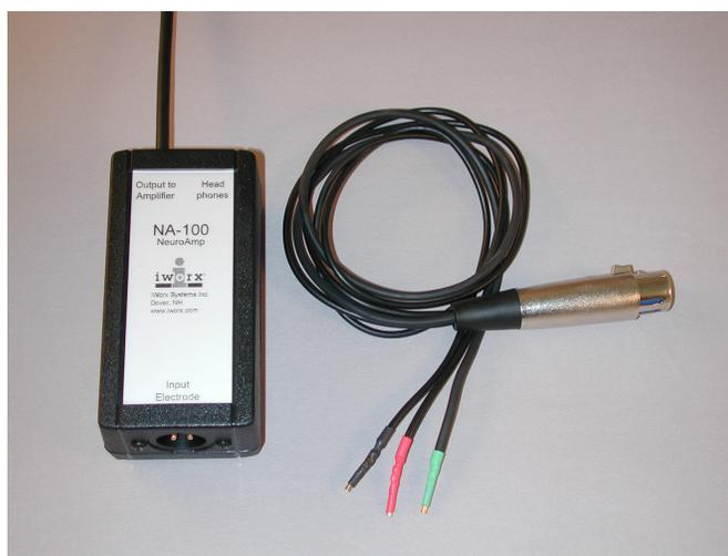
Figure AN-8-S1: The NA-100 Neuroamp Extracellular Amplifier and input cable.
