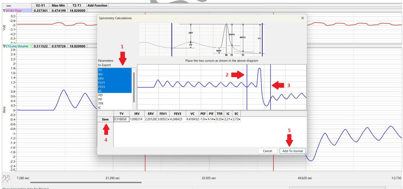
2. Move the blue vertical cursors so one is on the trough of the full regular breath before the big in/out breath and the 2<sup>nd</sup> is on the slight up-slope right after the trough of the big out breath. Refer to the image for placement of the cursors.
