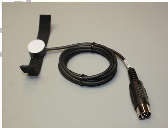
*Figure HP-14-S1: PT-104 pulse plethysmograph.*
