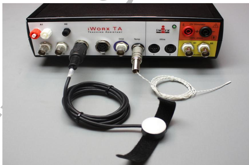
Figure HP-14-S6: The IXTA with the PT-104 and TM-220 plugged into the correct channels.
