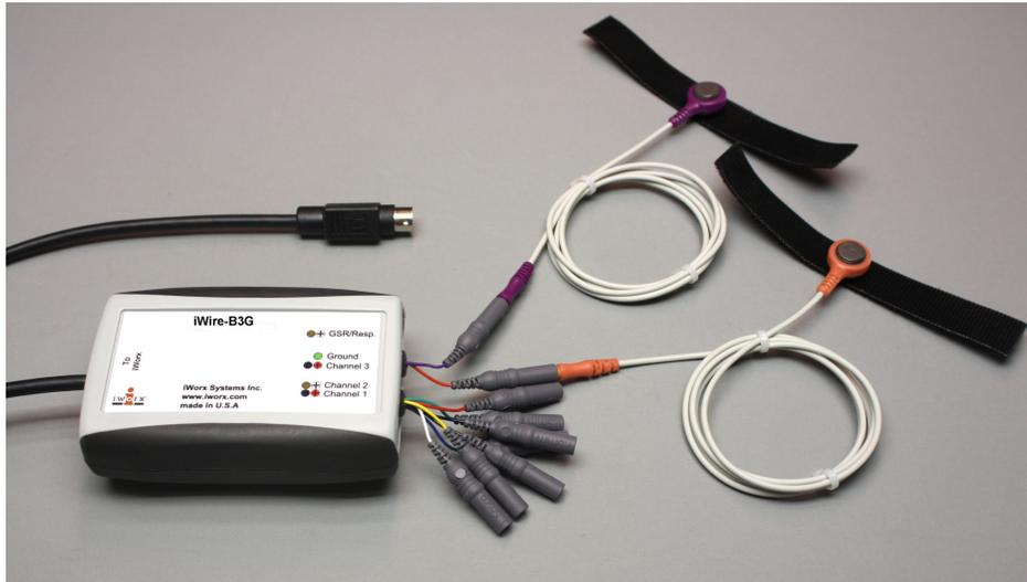
Figure HP-14-S2 The iWire-B3G ECG and Galvanic Skin Response amplifier. The purple and orange GSR electrodes are shown in this image.
