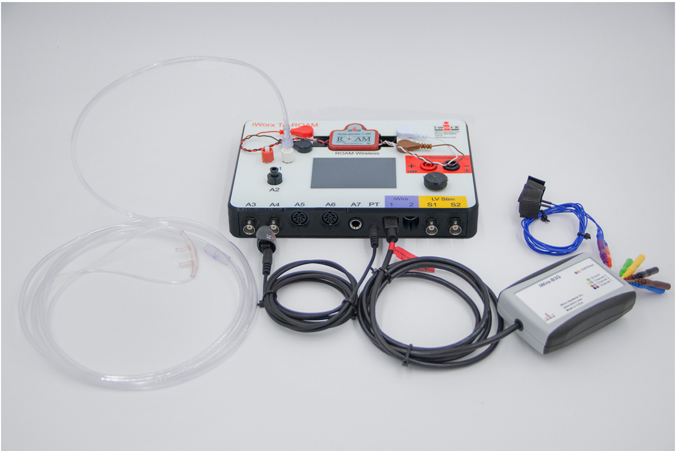
Figure HP-14-S1: PPG pulse plethysmograph, GSR and nasal cannula.
