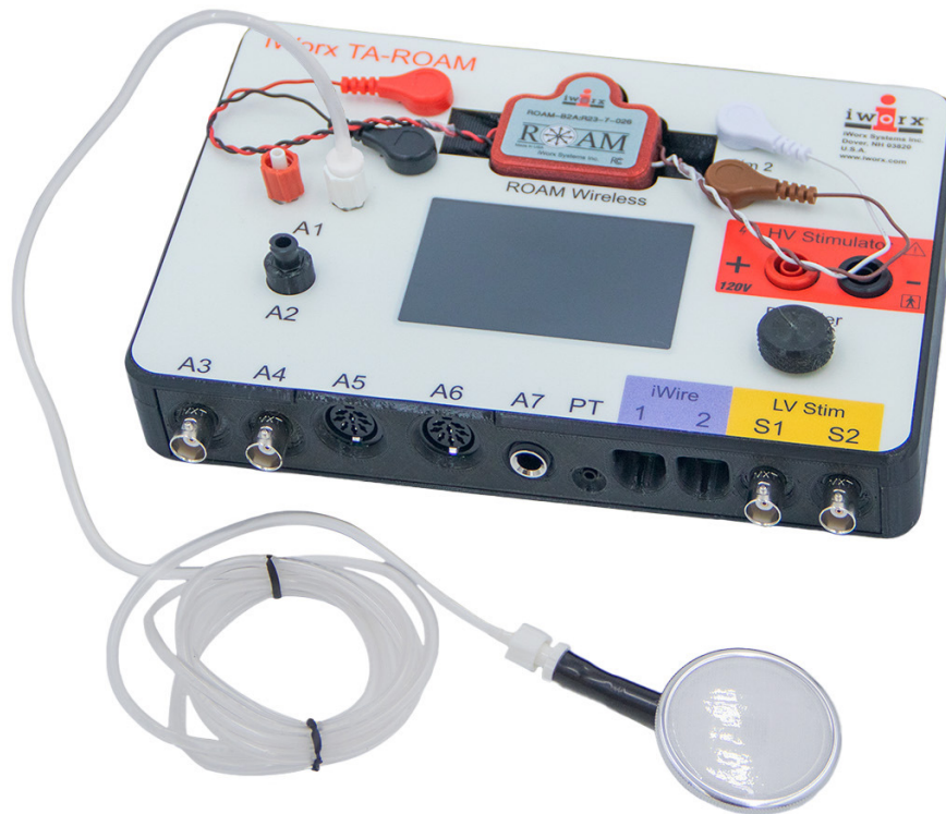
Figure HH-1-S1: The heart sounds microphone attached to the TA.
