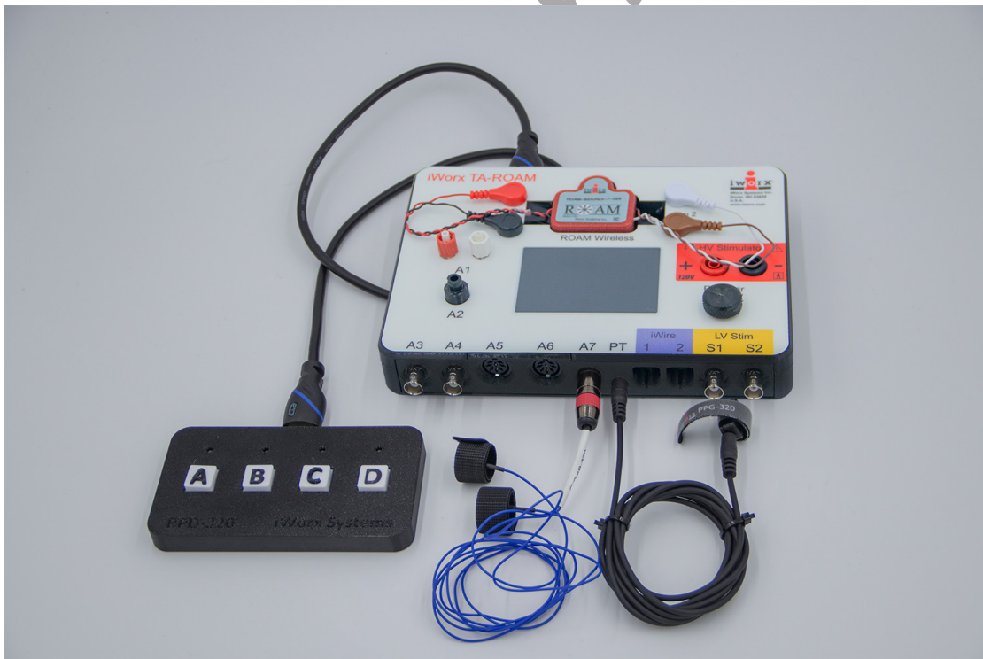
Figure HP-29-S1: The response pad, GSR and PPG sensor plugged into the TA.
