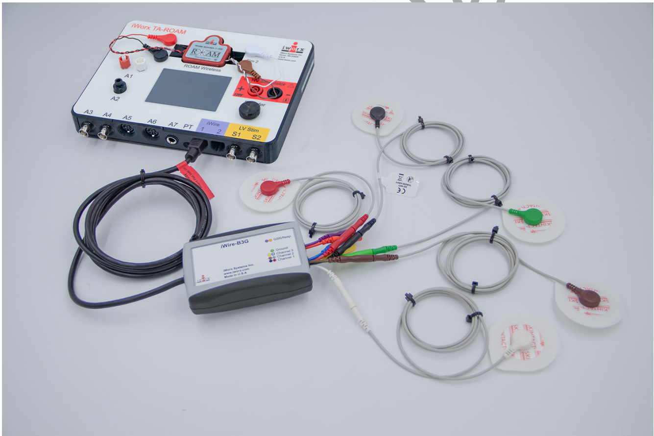
Figure HM-7-S2: A five lead EMG cable connected to the TA.
