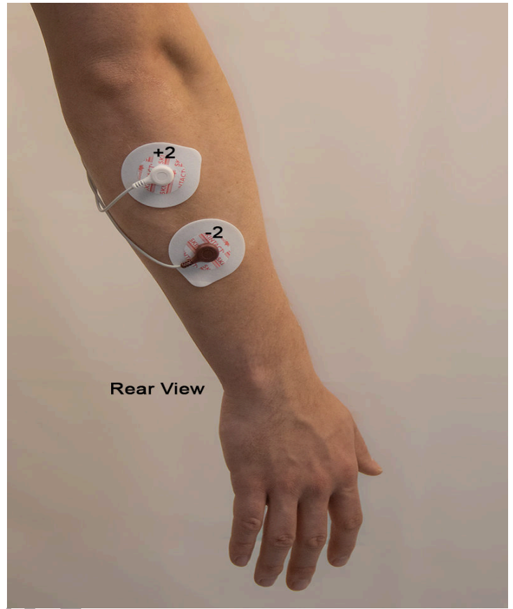
Figure HM-2-S2: Position of electrodes used to record EMG from muscles in the forearm during flexion and extension.
