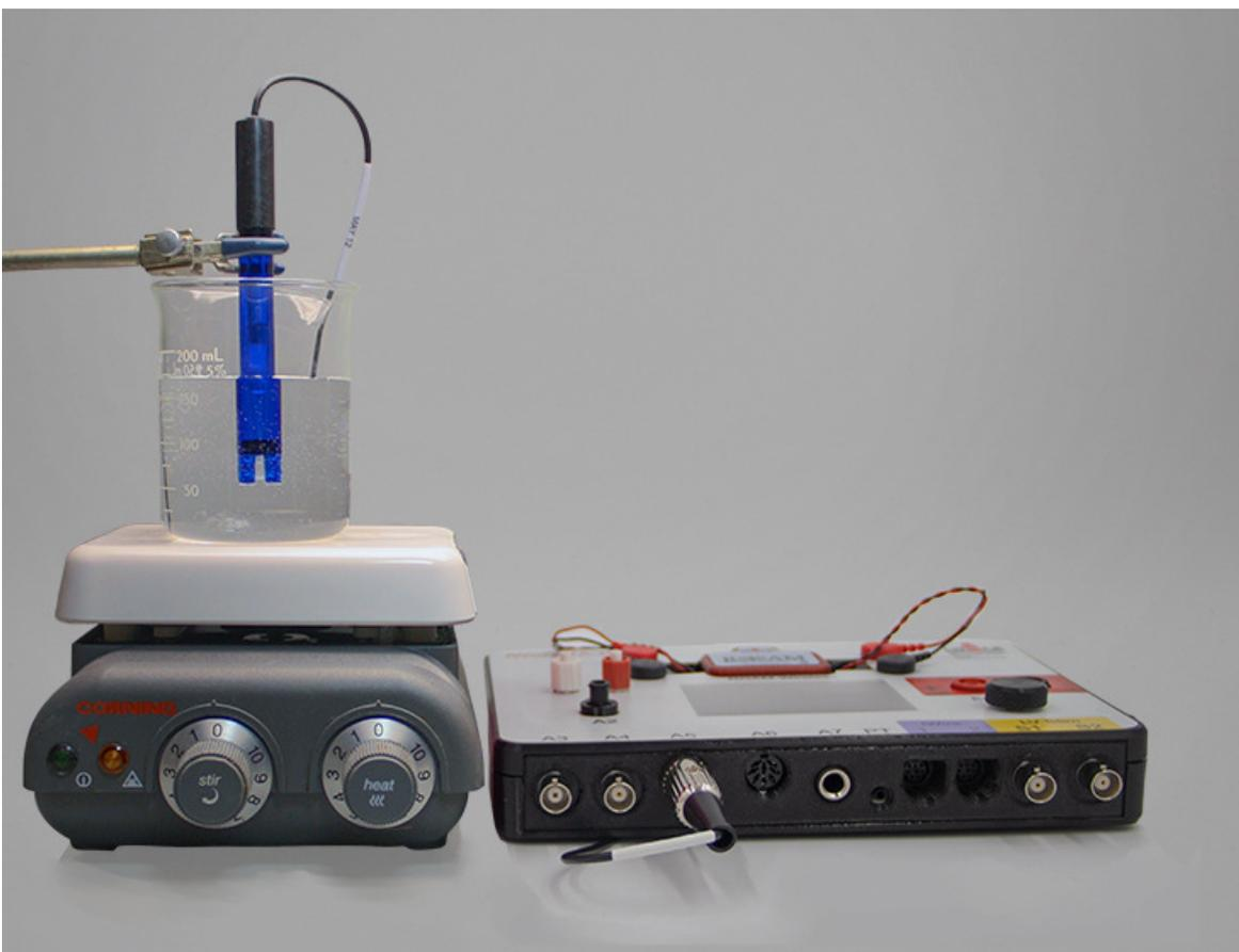
Figure GB-5-1: The arrangement of the stirrer, pH electrode, and beaker for the calibration of the pH probe.
