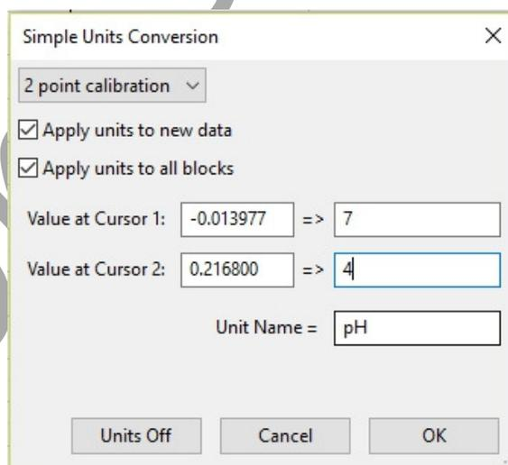
Figure GB-5-4: The Simple Units Conversion dialog window for pH conversion.
