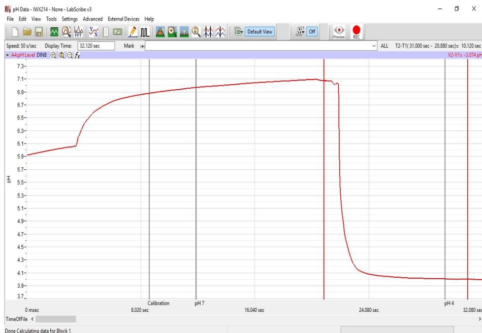
Figure GB-5-S3: pH calibration data recorded showing the positions of the cursors for changing the recorded voltage to pH values.
