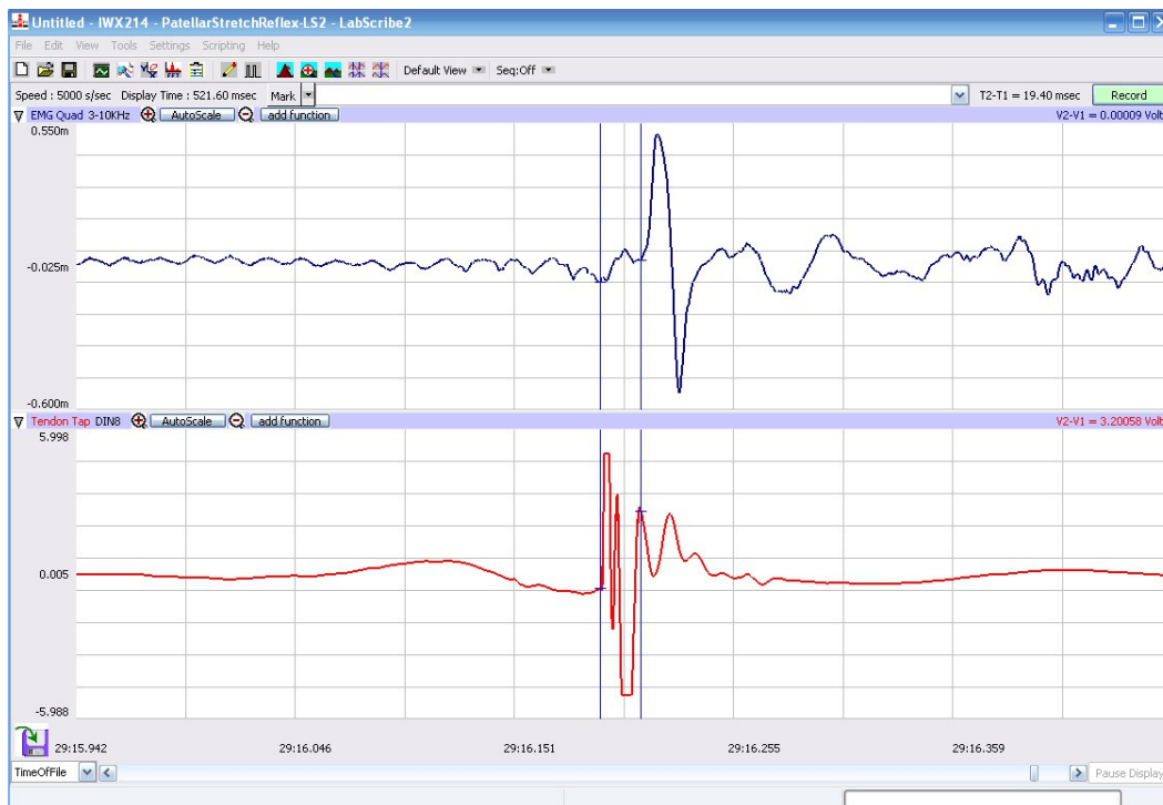
Figure NP-2-L1: An Achilles tendon reflex response and patellar hammer signal displayed on the Main window. The cursors are in position to measure the reflex conduction time
