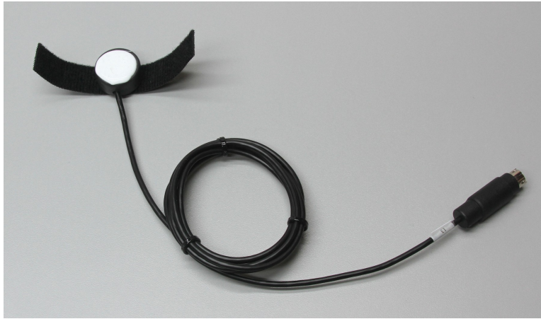
Figure NP-2-S1: The PT-104 pulse plethysmograph.
