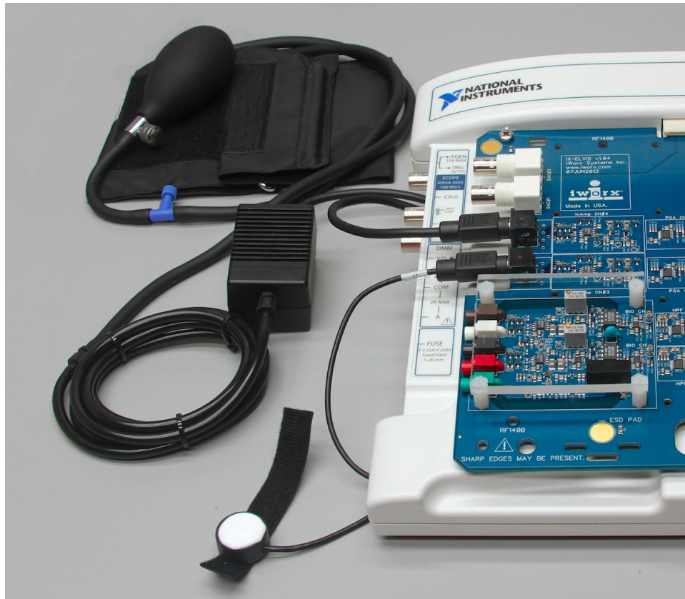
Figure VP-1-S3: The PTN-104 pulse transducer and the BP-220 non-invasive blood pressure transducer connected to the IX-ELVIS.
