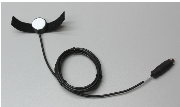
Figure VP-1-S2: The PTN-104 pulse plethysmograph.
