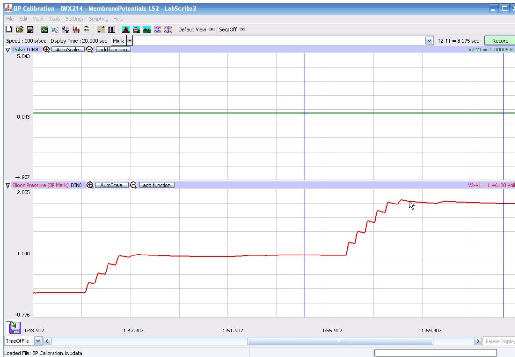
Figure VP-1-L1: The output of the BP-220 non-invasive blood pressure transducer displayed on the Main window with cursors at the points where the pressures in the cuff were 70 and 140 mmHg.
