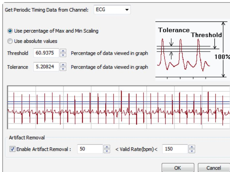
*Periodic dialog. Threshold is the amplitude value that will trigger detection of a beat. Tolerance determines the permissible range in amplitude for detection of a beat. Both are computed either as a percentage of the total amplitude of the data in the ECG or from absolute amplitude data values.*
