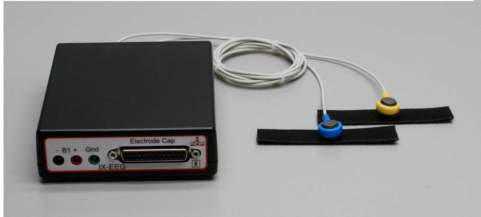
Figure HP-2-S1: The IX-EEG with GSR electrodes.
