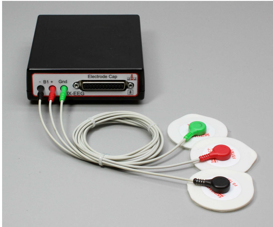
Figure HM-3-S1: The IX-EEG with three EGG lead wires and electrodes connected.
