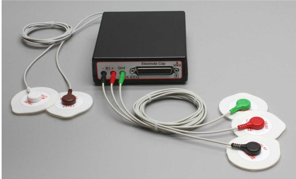
*Figure HH-4-S1: IX-EEG with five lead wires and electrodes connected.*
