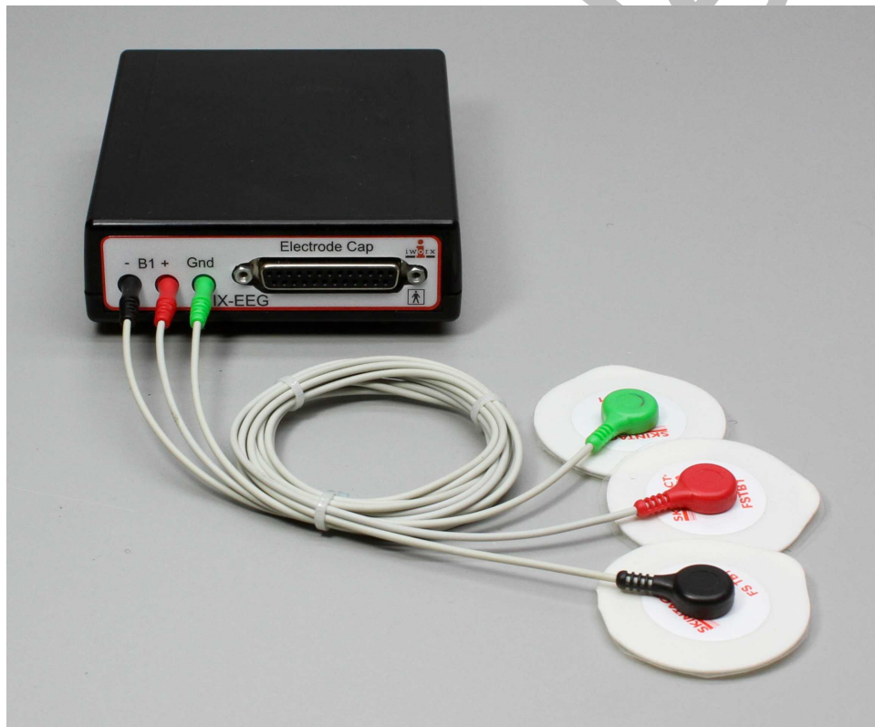
Figure HH-2-S1: The IX-EEG with three ECG lead wires and electrodes connected.
