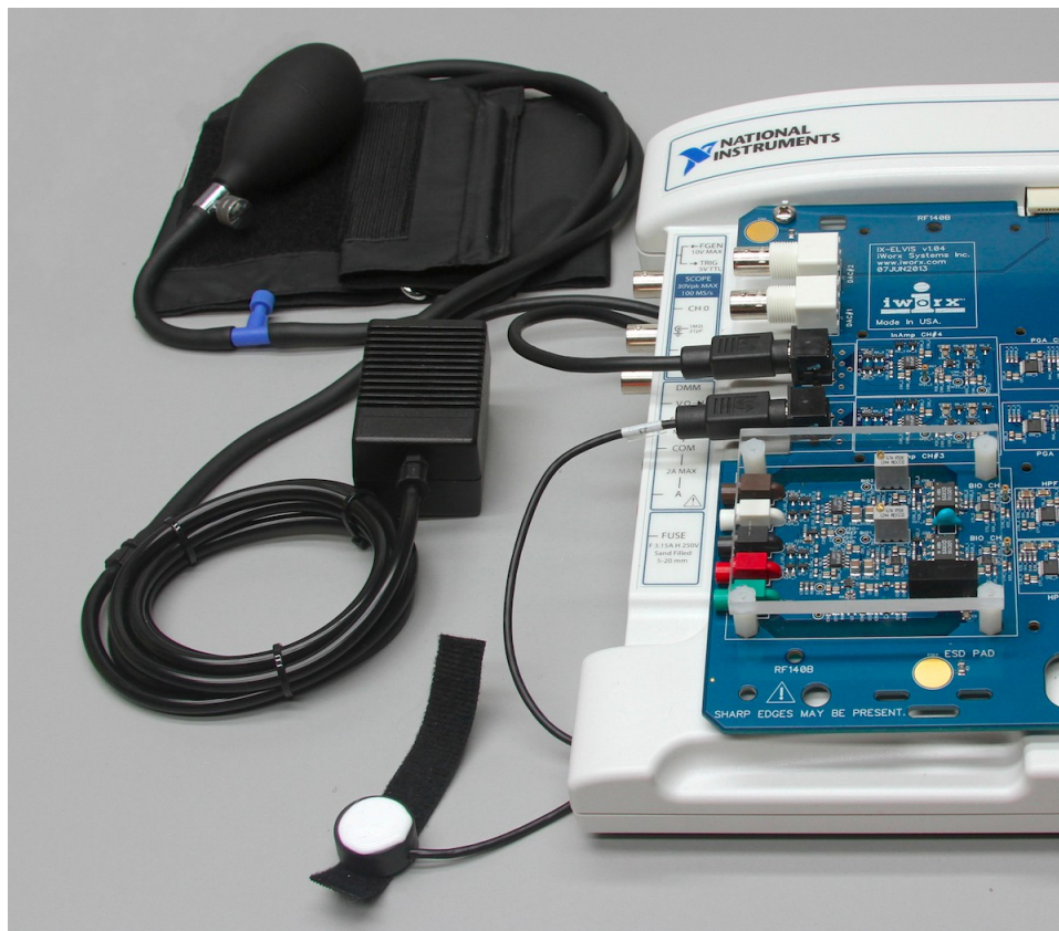
Figure VP-2-S3: The PTN-104 pulse transducer and the BP-220 non-invasive blood pressure transducer connected to the IX-ELVIS.
